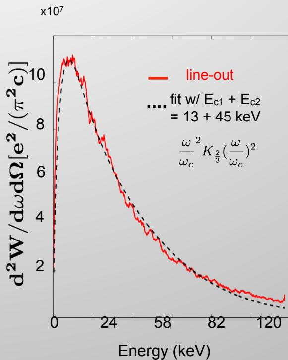
**Spectrum fitted with synchrotron spectrum with critical photon energies of 13 and 45 KV respectively, emitted by two groups of electrons with similar energies but very different initial radii.**
