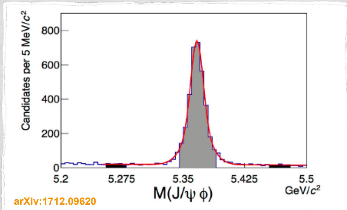
3.5k signal  $B^0_s \rightarrow J/\psi(\rightarrow \mu\mu)\phi(\rightarrow KK)$  decays
