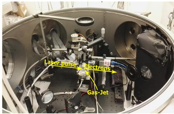
The gas, transported by the gas-jet, is synchronously injected with the laser pulse, that stimulates the plasma wakefield, so that an electron bunch in the same direction of the laser is generated.
