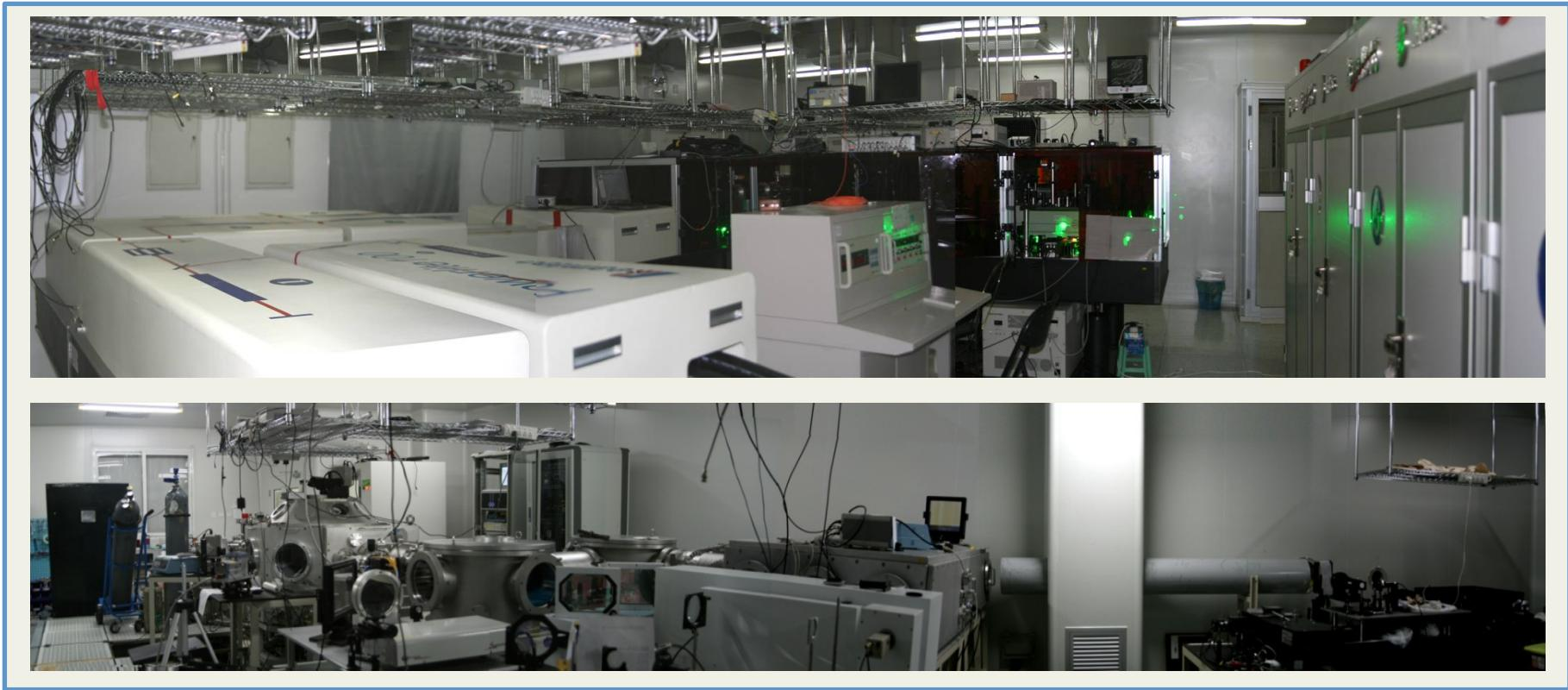
**20TW/100TW/1PW systems with 3 target chamber**
