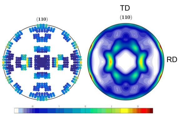
21 diffraction measurements covered a quarter of pole figure. It is complemented with ODF (mtex-4.0.12) 14
