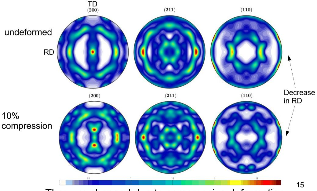
They are changed due to compressive deformation
