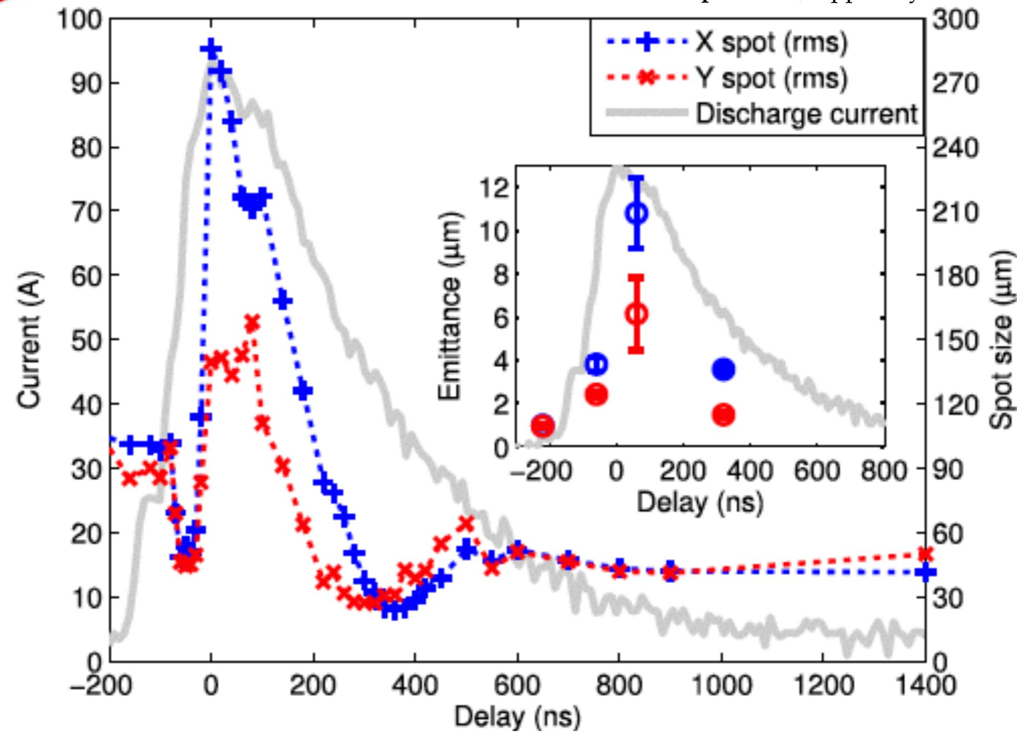
The arrival time of the electron beam is scanned with respect to the discharge pulse in order to change the active plasma lens focusing.
