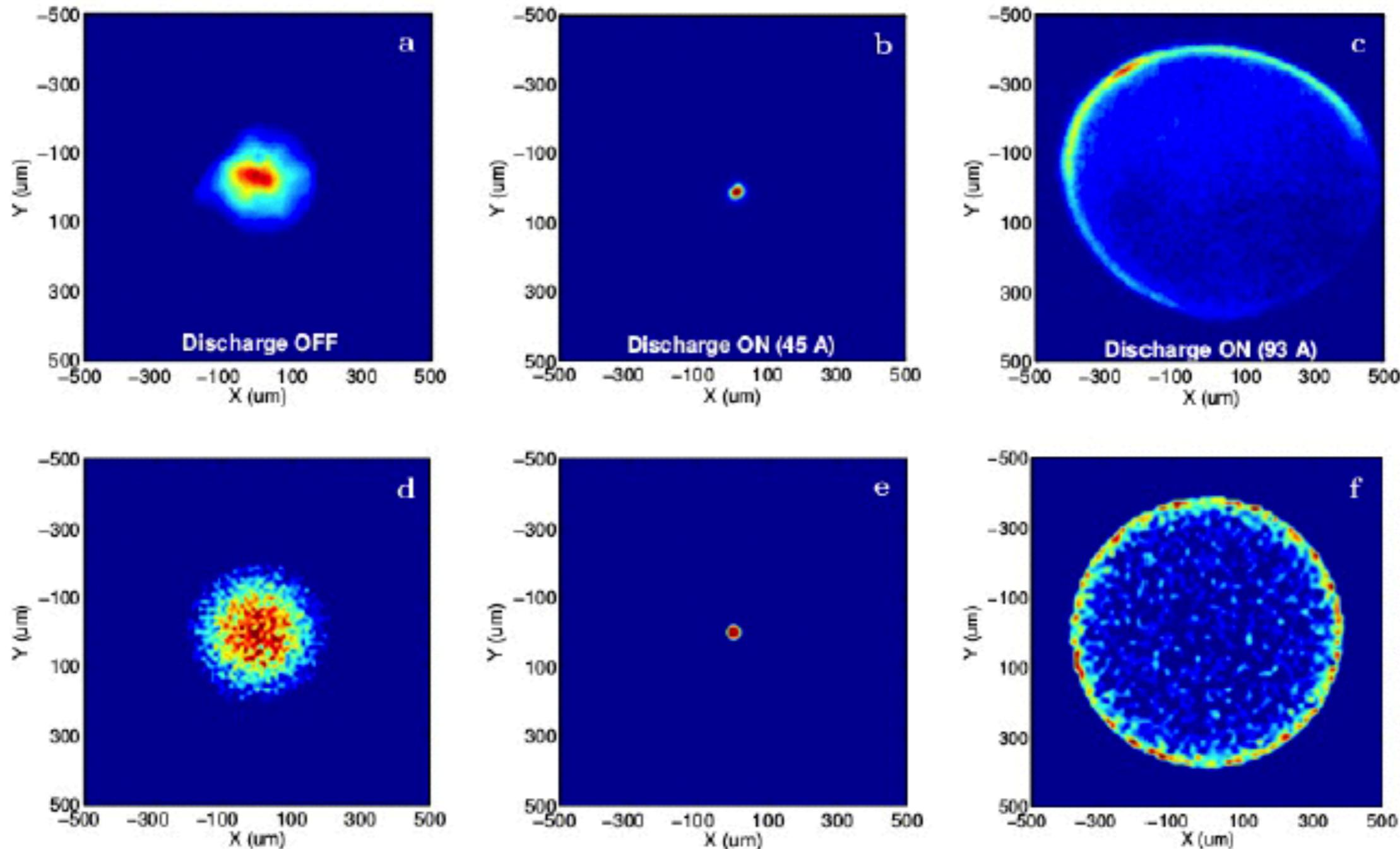
Images recorded on the screen downstream the capillary with the discharge turned off ( $\sigma \approx 100 \mu\text{m}$ , a) and on, at  $\text{ID} \approx 45 \text{ A}$  ( $\sigma \approx 24 \mu\text{m}$ , b) and  $\text{ID} \approx 93 \text{ A}$  ( $\sigma \approx 280 \mu\text{m}$ , c). (d-f) Simulated transverse profiles obtained on the same screen with the combined use of the GPT and Architect codes.
