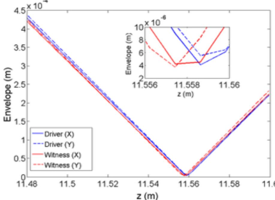
GPT simulation for the final focus with PMQ from experimental beam parameters
