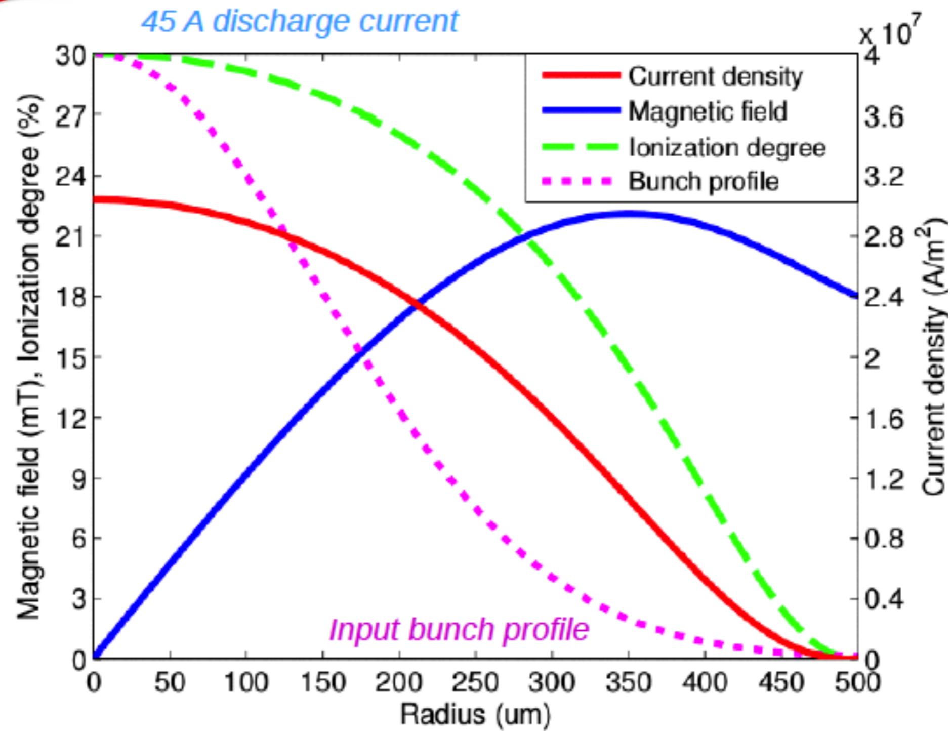
The current flows mainly on the axis and thus resulting in a radially nonlinear magnetic field
