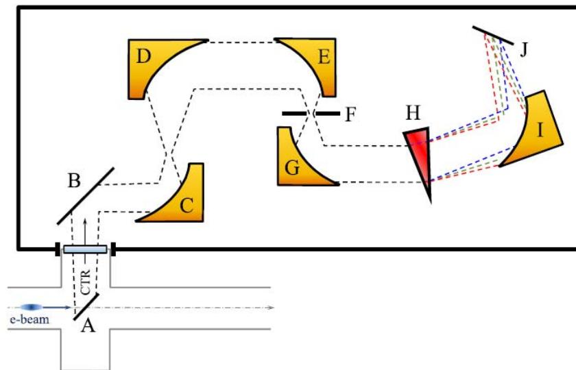
KRS-5 (thallium bromoiodide) prism based spectrometer developed
