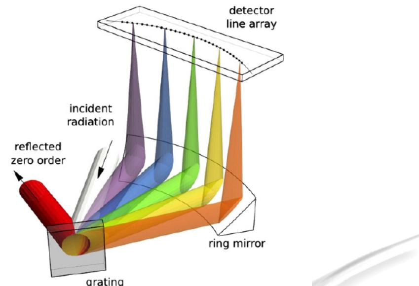
Pyro-electric line detector 30 channels @ room temperature no window, works in vacuum fast read out sensitivity
