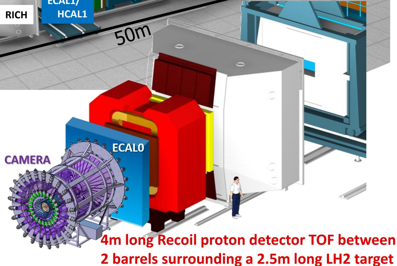
4m long Recoil proton detector TOF between 2 barrels surrounding a 2.5m long LH2 target
