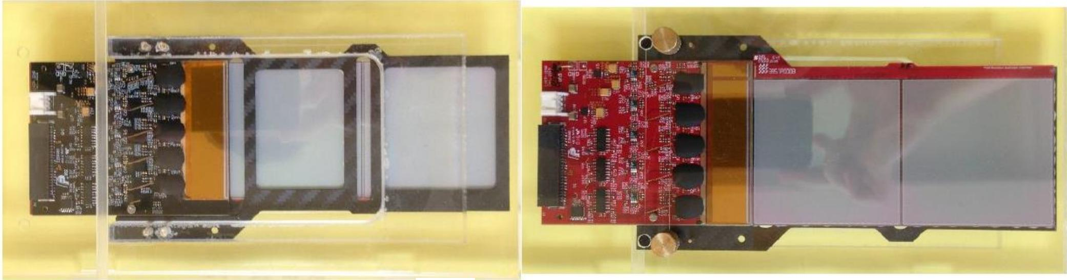
The Silicon detector unit developed for BM@N experiment at NICA. The unit contains electronics for 640 strips. The front-end electronics is based on a charge sensitive preamplifier chip VTAGP7 (IDEAS)
