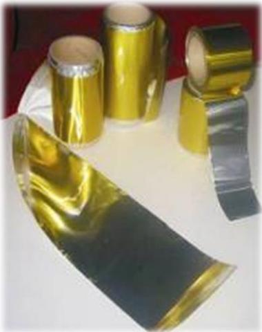
Long flat aluminium-polyimide multilayer flexible buses (thickness  $< 50 \mu\text{m}$ )
