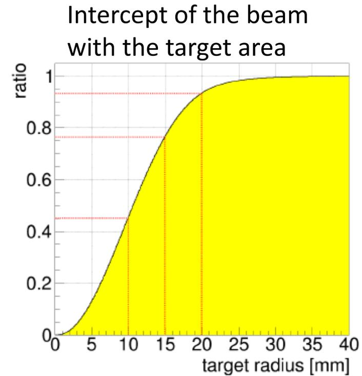
It could be worth to reduce the beam intercept with a target radius of 15mm to reach smaller  $t_{min}$
