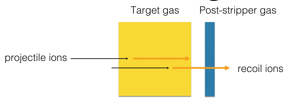
The use of an additional layer of a different gas can make charge state independent of reaction coordinate within the target
