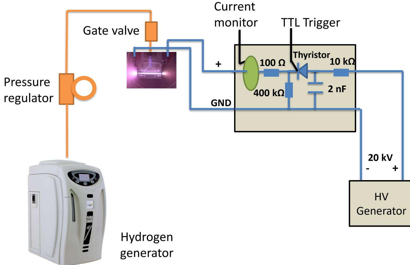
High voltage is stored into a capacitor until a TTL signal triggers the thyristor letting the current flow into the gas.
