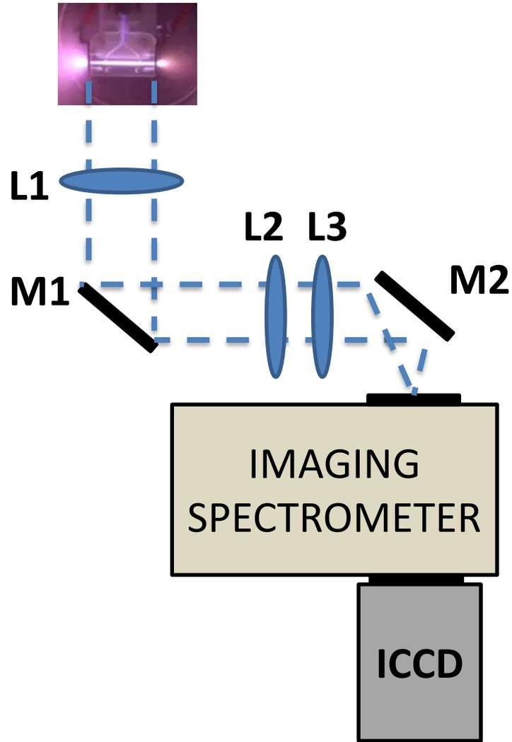
A system of lenses collects the self-emitted light of the capillary and image it onto the spectrometer slit.
