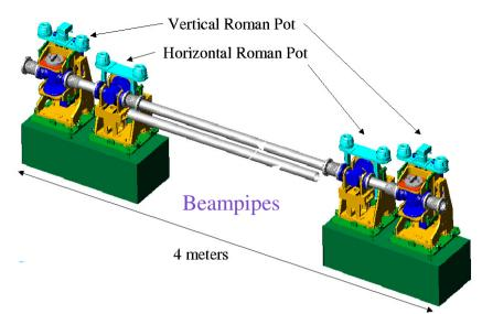
Each RP station has 2 units, ~5m apart. Each unit has 3 insertions ('pots'): 2 vertical and 1 horizontal
