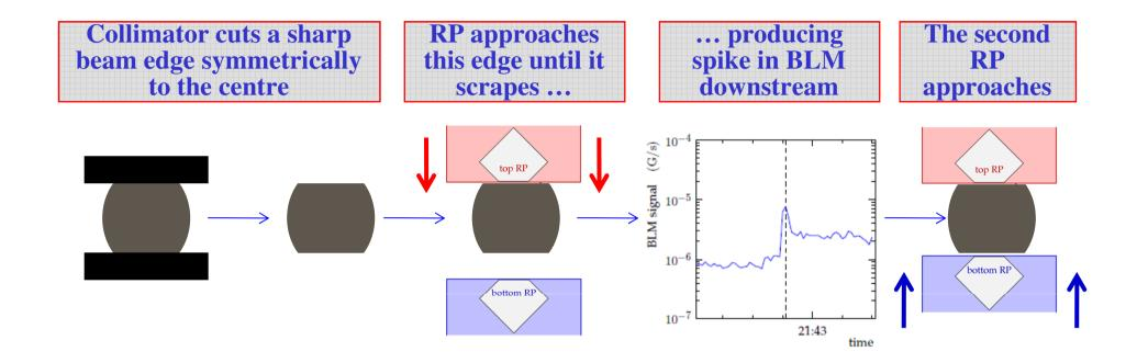
When both top and bottom pots "feel" the edge: they are at the same number of sigmas from the beam centre as the collimator and the beam centre is exactly in the middle between top and bottom pot
