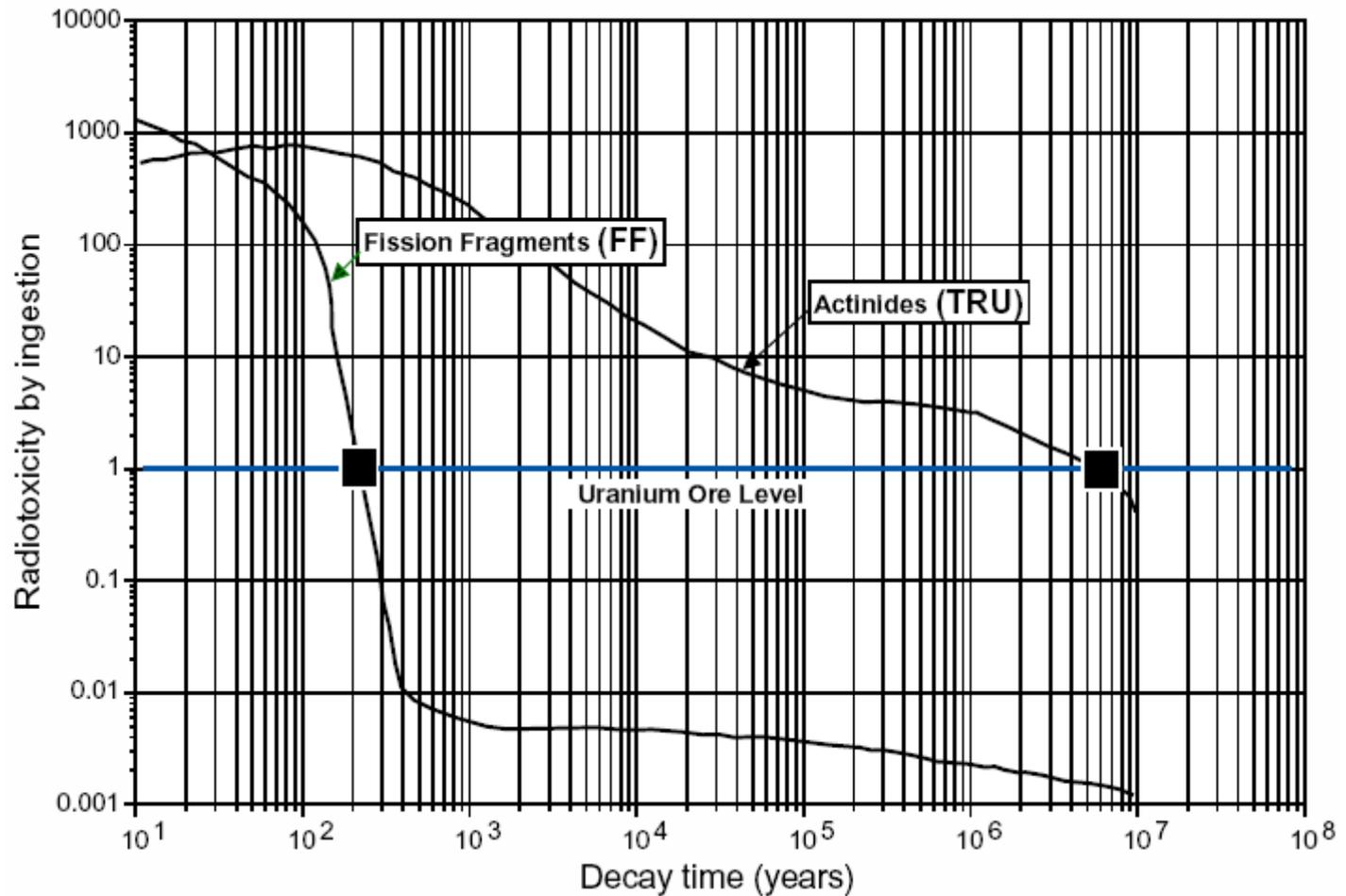
**Time evolution of the potential radio-toxicity (relative to uranium ore) of the two main components of nuclear waste for PWR spent fuel.**
