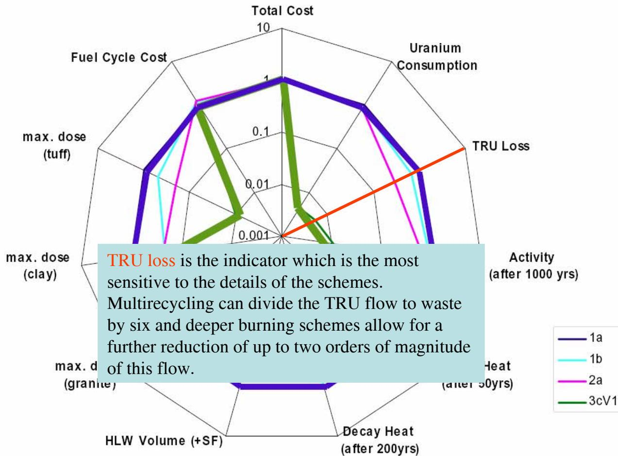
TRU loss is the indicator which is the most sensitive to the details of the schemes. Multirecycling can divide the TRU flow to waste by six and deeper burning schemes allow for a further reduction of up to two orders of magnitude of this flow.
