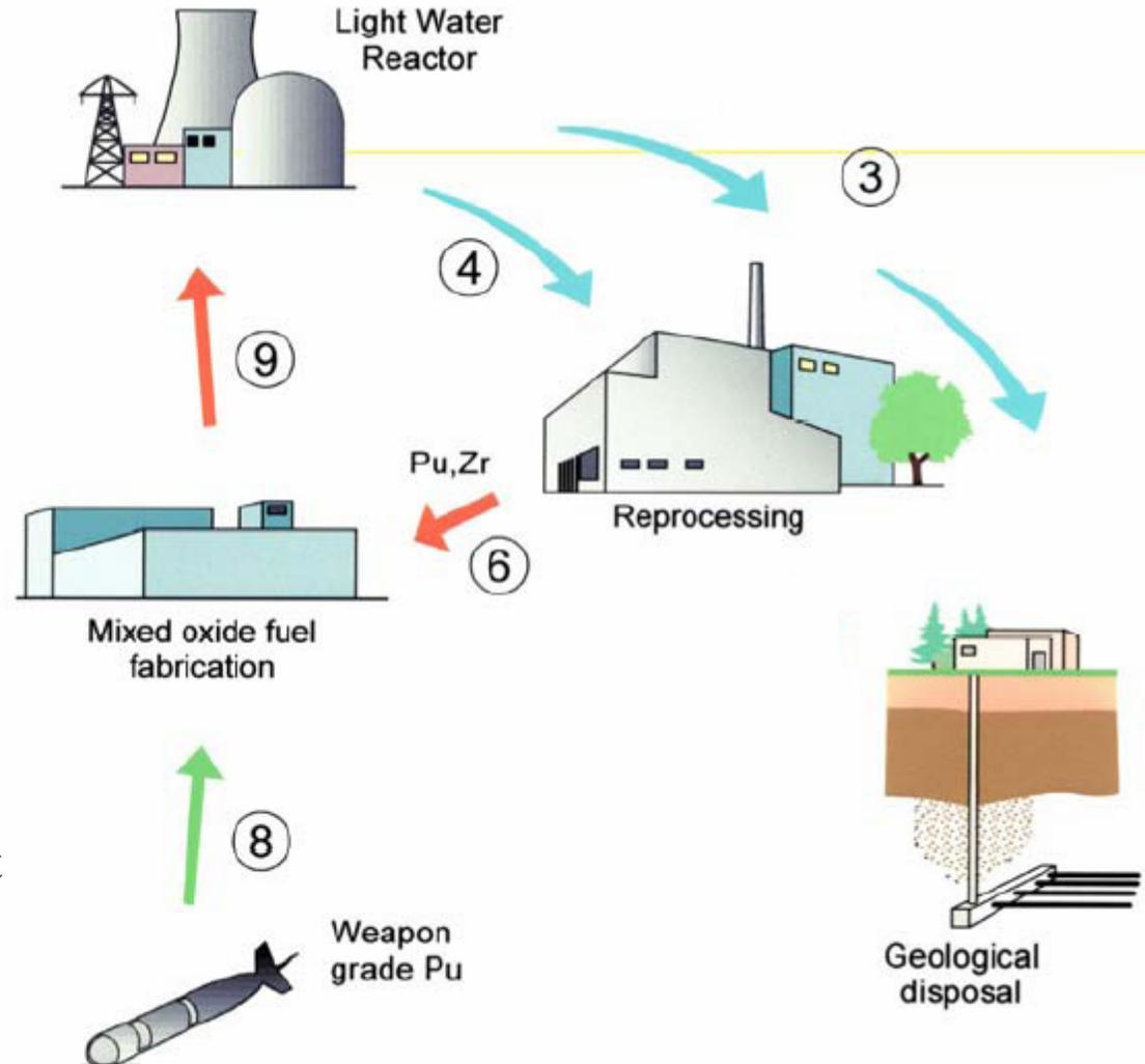
Fuel cycle extension. It includes spent U-fuel reprocessing, plutonium fuel fabrication (U-free), Pu burning in the reactor, intermediate storage and direct geological disposal of the rock-like spent fuel.
