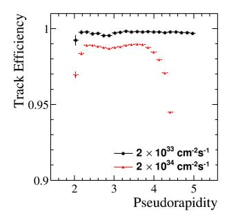
Tracking efficiency reduced to 96% (not so bad) + less flat
