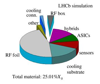
Significant and immediate physics gain from removing the RF foil
