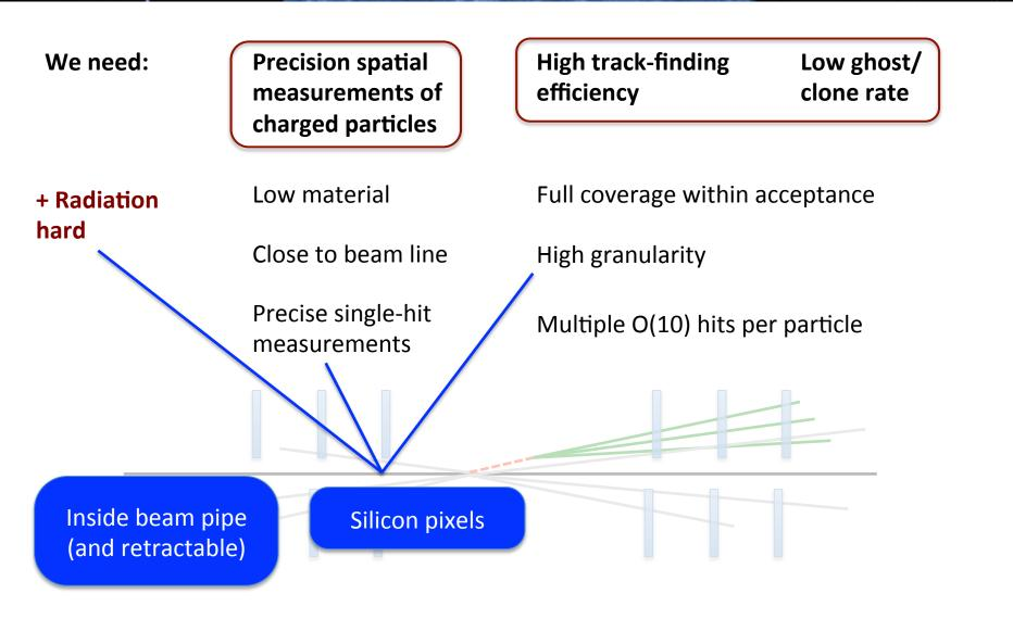
**Precision spatial High track-finding** Low ghost/ We need: measurements of efficiency clone rate charged particles Low material Full coverage within acceptance + Radiation hard Close to beam line High granularity Precise single-hit Multiple O(10) hits per particle measurements High read-out rate Inside beam pipe Silicon pixels (and retractable) High performance, low material cooling
