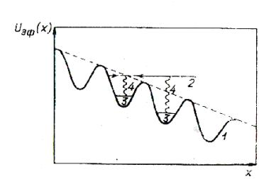
Volume capture of fast charged particles in a bent crystal
