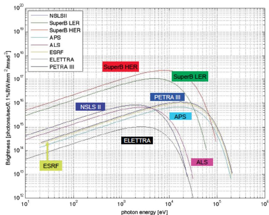
Figure 1: Brightness generated from bend magnets as a function of photon energy.
