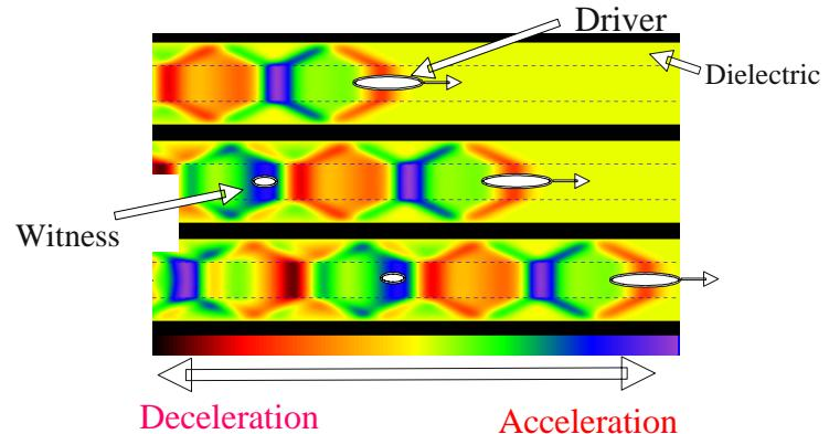
Longitudinal and radial components of electric and magnetic fields in the cross-section
