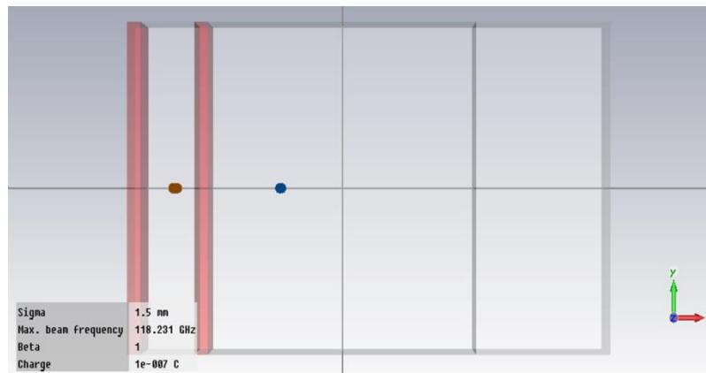
a train of  $4 \times 75$  MeV bunches of 25 nC each. Structure parameters are: **a=375 um, c= 2.1 mm, d=2.85 mm** ; dielectric permittivity of the inner tube  **$\epsilon=35.7$**  and of the outer layer  **$\epsilon= 5.7$** .
