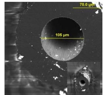
Diamond, single crystal, 427  $\mu\text{m}$  ID, 755  $\mu\text{m}$ , 3.99 mm;
