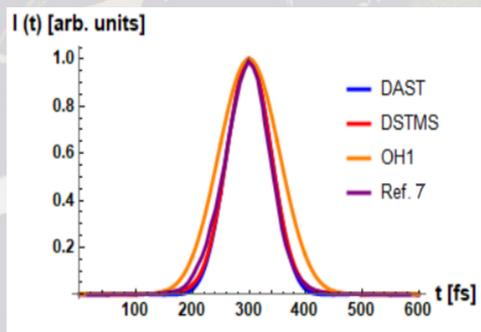
An almost perfect matching between the pump pulse envelope as measured in [6,7] with the envelope retrieved by our technique can be obtained exploiting DAST (180μm) and DSTMS (900 μm) crystals; FWHM: 95±15 fs, in agreement with the temporal duration measured in [7]. The FWHM of the pump laser as retrieved when considering the OH1 (440 μm) THz spectrum was 126±21 fs. Our methodology allows to retrieve the phase of the pump pulse.
