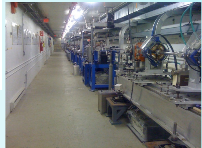
LEUTL tunnel is ~ 40 m long and is ready to accept the beam
