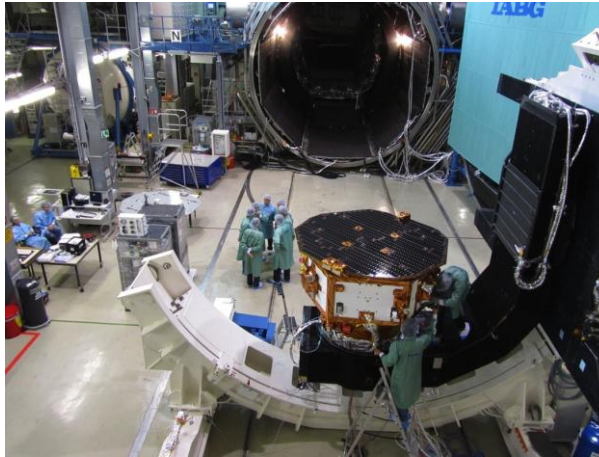
Spacecraft + optical bench tests
