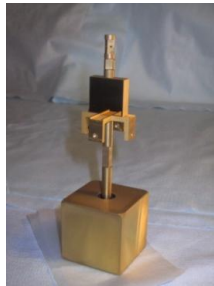
1-mass torsion pendulum (torques)
