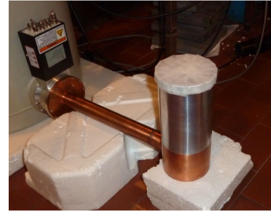
The Os sample as it should be installed on the BEGe detector
