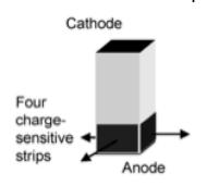
Reduces number of channels required while retaining good energy resolution.
