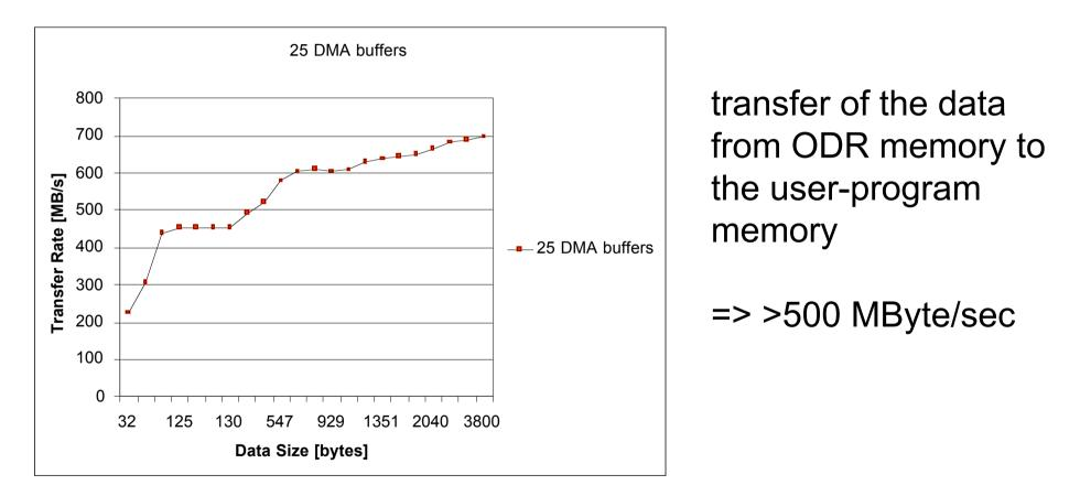
All measurements: single requester thread, no disk write, data copied To the host memory.
