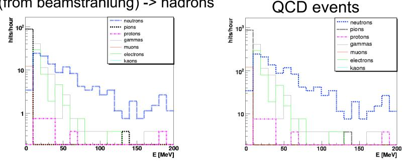
$\Rightarrow$  SEU rate of 14 min-12hours depending on FPGA type for the whole ECAL, needs to be taken into account in control software  $\Rightarrow$  fluence of 2\*10<sup>6</sup>/cm per year, not critical  $\Rightarrow$  radiation of 0.16Rad/year, not critical
