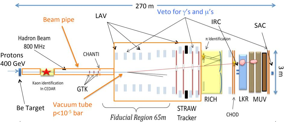
3 × 10<sup>12</sup> ppp, 750 MHz on beam spectrometer (6% K+), ~10 MHz downstream, O(10 KHz) final trigger rate
