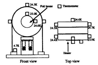
Fig. 3. Distribution of the equilibrium temperature in the case of 29 mW heat power.
