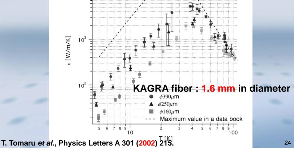
Thick sapphire fibers (about 1.6 mm in diameter) with nail heads are necessary to suspend mirrors. Test sample (T. Uchiyama)
