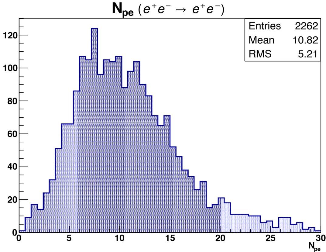
Amplitude spectrum of the THICK system
