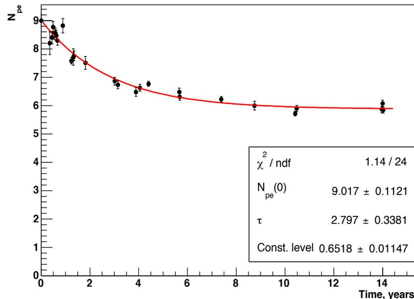
*Dynamic of the amplitude dependence on time is explained by slow aerogel degradation which goes to some stable level.*
