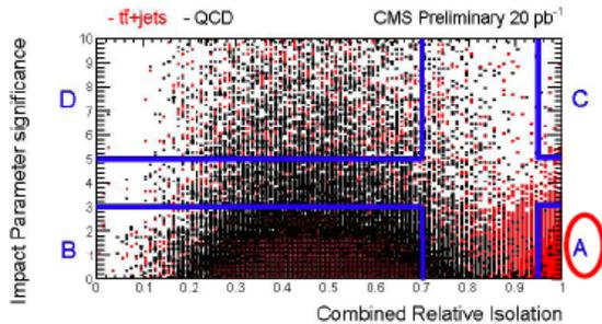
Figure 2. ABCD method used to estimate the QCD multi-jet background in the muon+jets channel.
