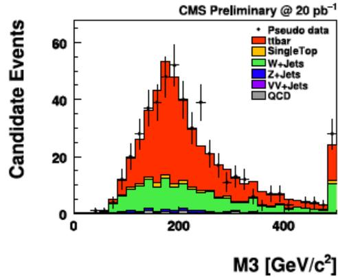
Figure 3.  $M3$  distribution : invariant mass of the three jets leading to the highest invariant mass (muon+jets channel).
