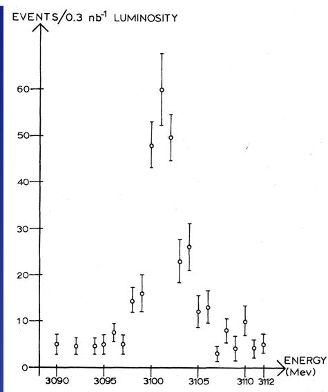
FIG. 1. Result from the Gamma-Gamma Group, total of 446 events. The number of events per  $0.3 \text{ nb}^{-1}$ luminosity is plotted versus the total c.m. energy of the machine. Volume 53B, number 4
