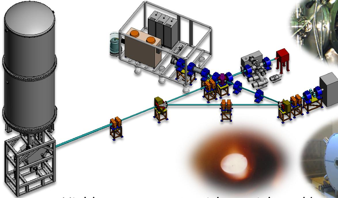
Yield measurements with particle and/or gamma detector arrangements
