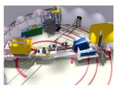
Hall C: High momentum spectromer and Short Orbit Spectrometer—well-controlled acceptance for precise cross section measurements
