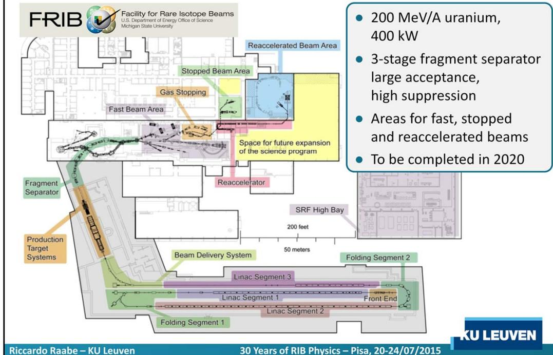
The FRIB at MSU will provide beams at most energy ranges.
