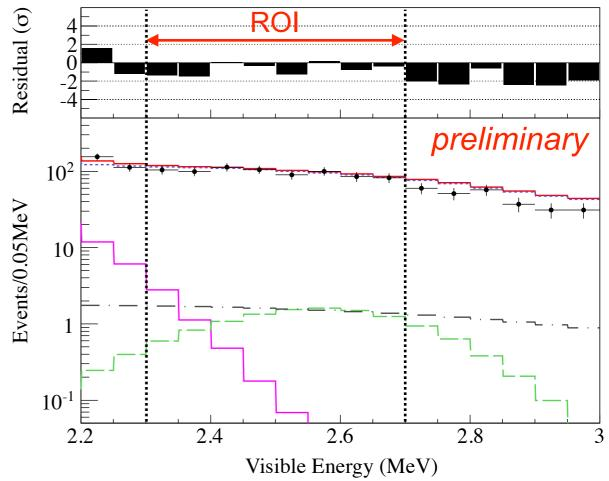
Fit to Energy-Volume 2D spectra Limits on 0vββ at 90% C.L. < 17.0 events/day/kton-LS  $\downarrow_{T^{0v}_{1/2} > 1.3 \times 10^{25} \text{ yr}}$
