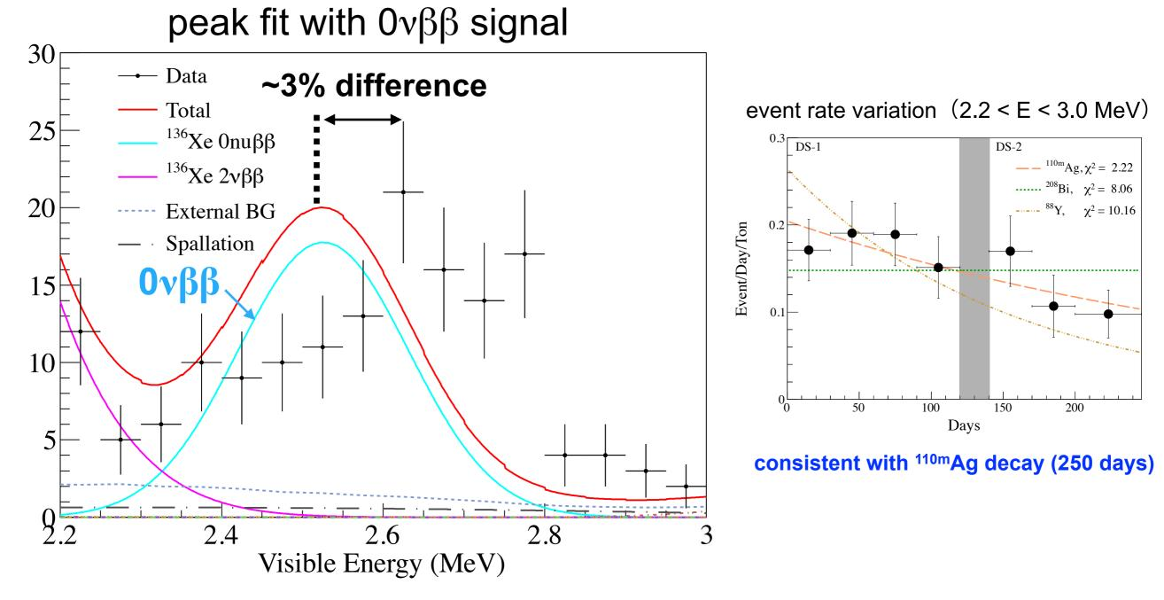
different peak position and time variation in event rate  $^{136}$ Xe  $0v\beta\beta$  only is rejected at more than  $8\sigma$  level
