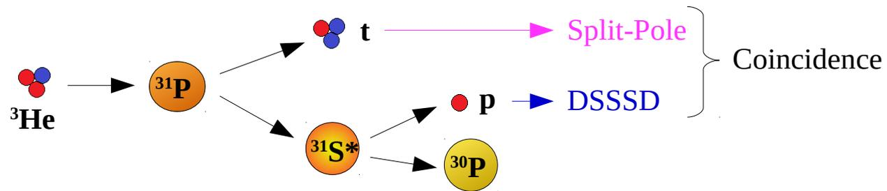
✓ Set-up: Split-Pole (SP) magnetic spectrometer + Double Sided Silicon Strip Detector (DSSSD) array:
