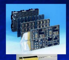
PICsIT module & CsI crystal glued to its photodiode
