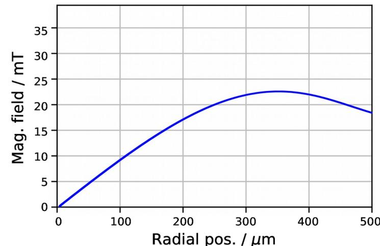
Magnetic field expected after 450ns from the start of the discharge from analysis of Sparc electron beam\*.
