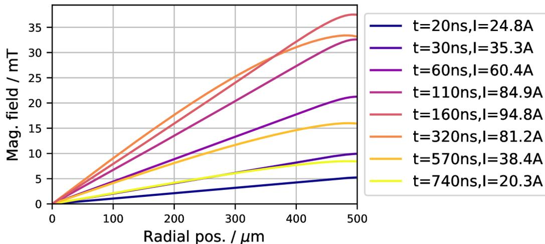
Computed magnetic field at different times in 1D simulation.
