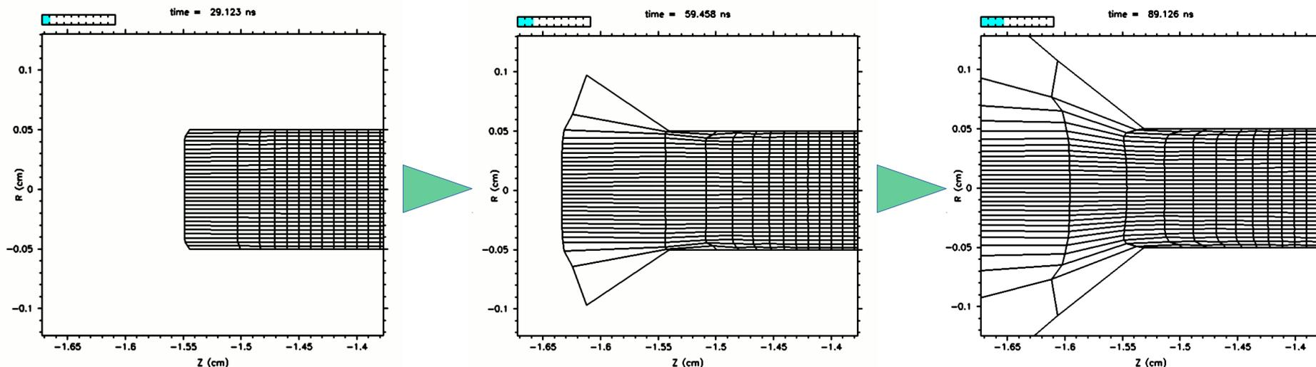
Typical evolution of the mesh in a hydrodynamic simulation (with DUED)
