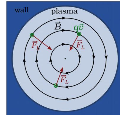
Schematic transverse view of an active plasma lens
