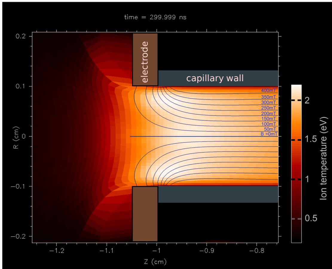
Particular of the plasma temperature (colored map) and azimuthal magnetic field (contour lines) in proximity of the left electrode at 300ns from the start of the discharge.
