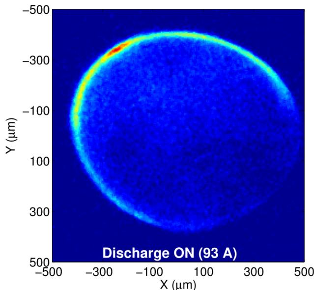
Beam spot 20cm downstream the active lens, operating at 93A\*.
