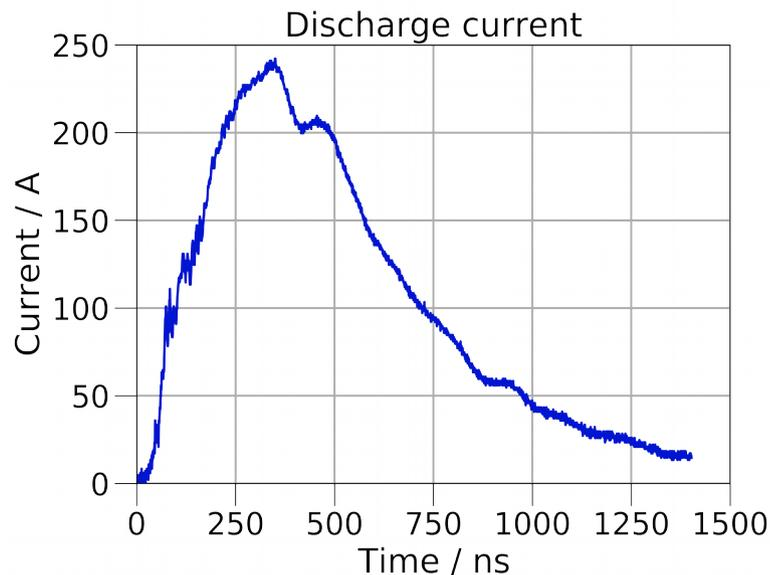
Example of time profile of the current during a discharge
