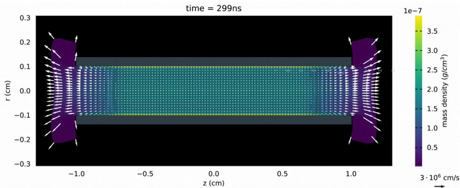
Mass density map and velocity field of the gas flowing from the capillary at 300ns from the start of the discharge.
