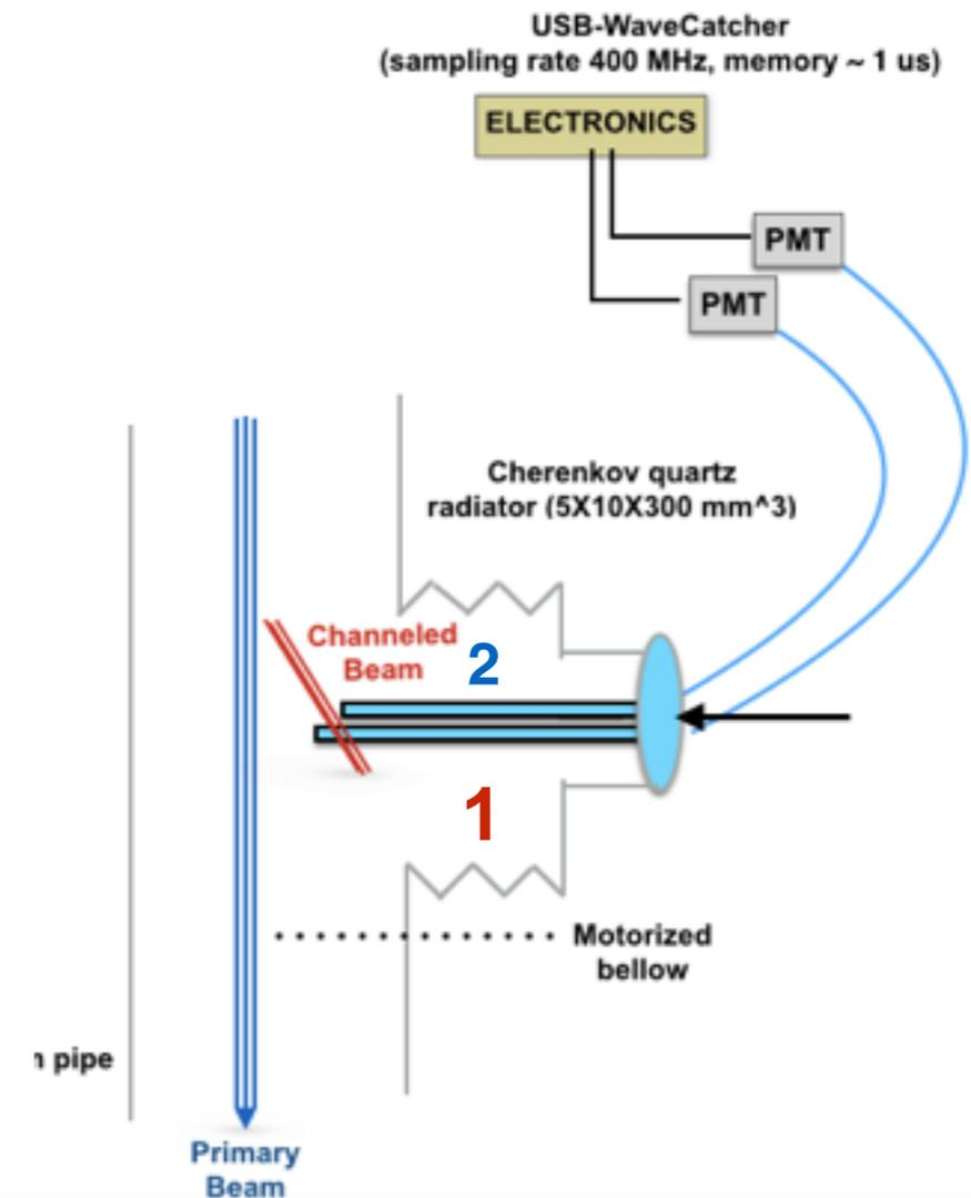
UA9 Crystal as a primary collimator. As the bars approach the channeled beam, the amplitude of the signal increases, until the channeled beam is fully intercepted. Moving the bars further, the first one touches the edge of the primary beam.
