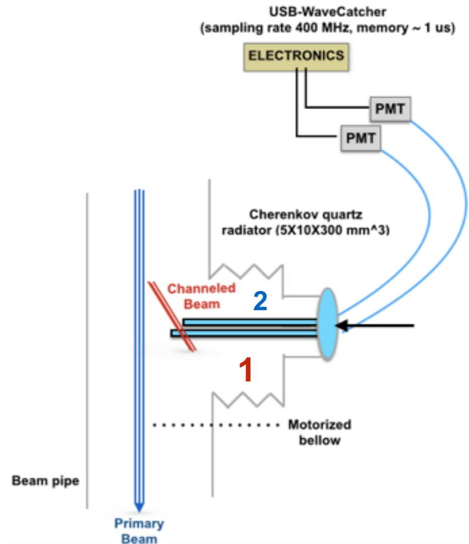
UA9 Crystal as a primary collimator. As the bars approach the channeled beam, the amplitude of the signal increases, until the channeled beam is fully intercepted. Moving the bars further, the first one touches the edge of the primary beam. The shift of the fit peaks is due to the relative shift of the bars (5,5 mm)
