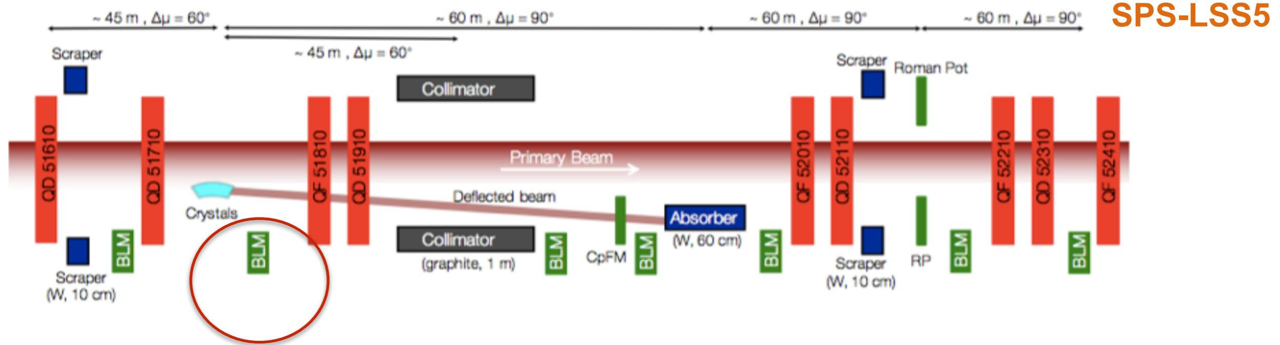
Channeling efficiency up to 80% in circulating beam (considering also multi-turn effect)
