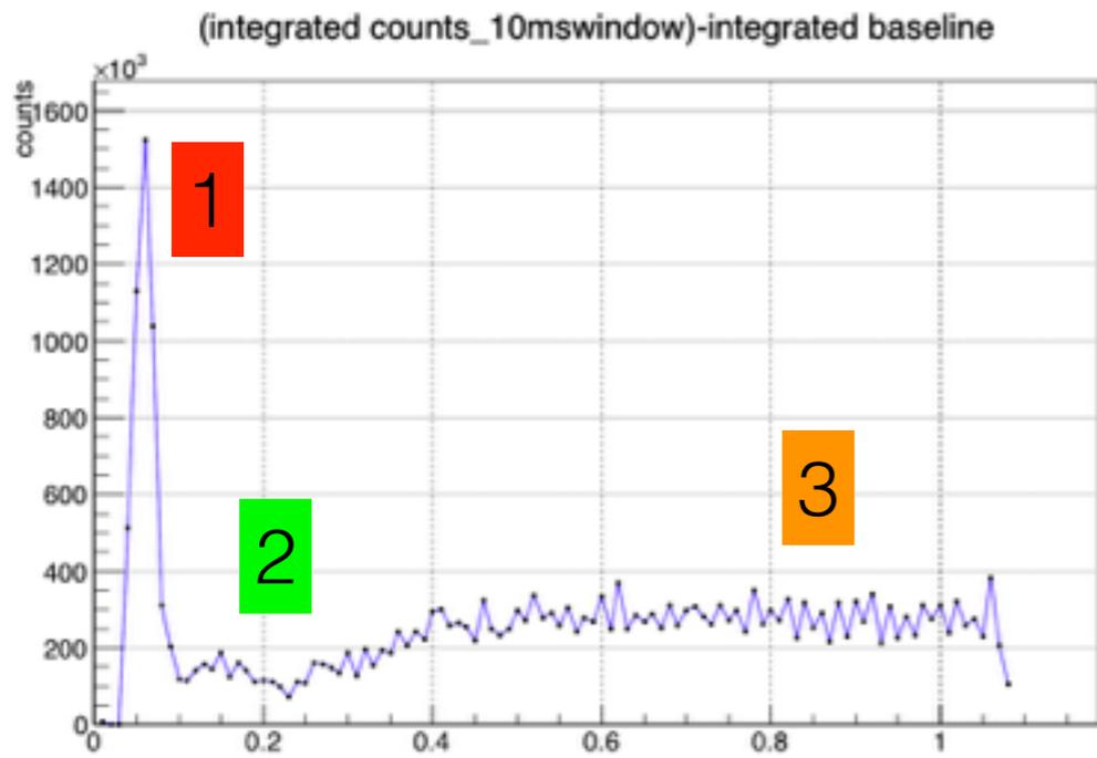
integrated digitized signal in time window of 10 ms, for 1 sec of spill: Is it clearly visible a huge intensity spike at the beginning of the spill. After first 400ms, as expected, the intensity becomes quite stable
