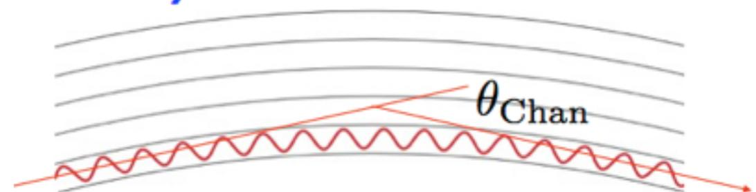
4 mm Si Crystal with a bending angle of 50urad produces the same kick of a 310T magnet!
