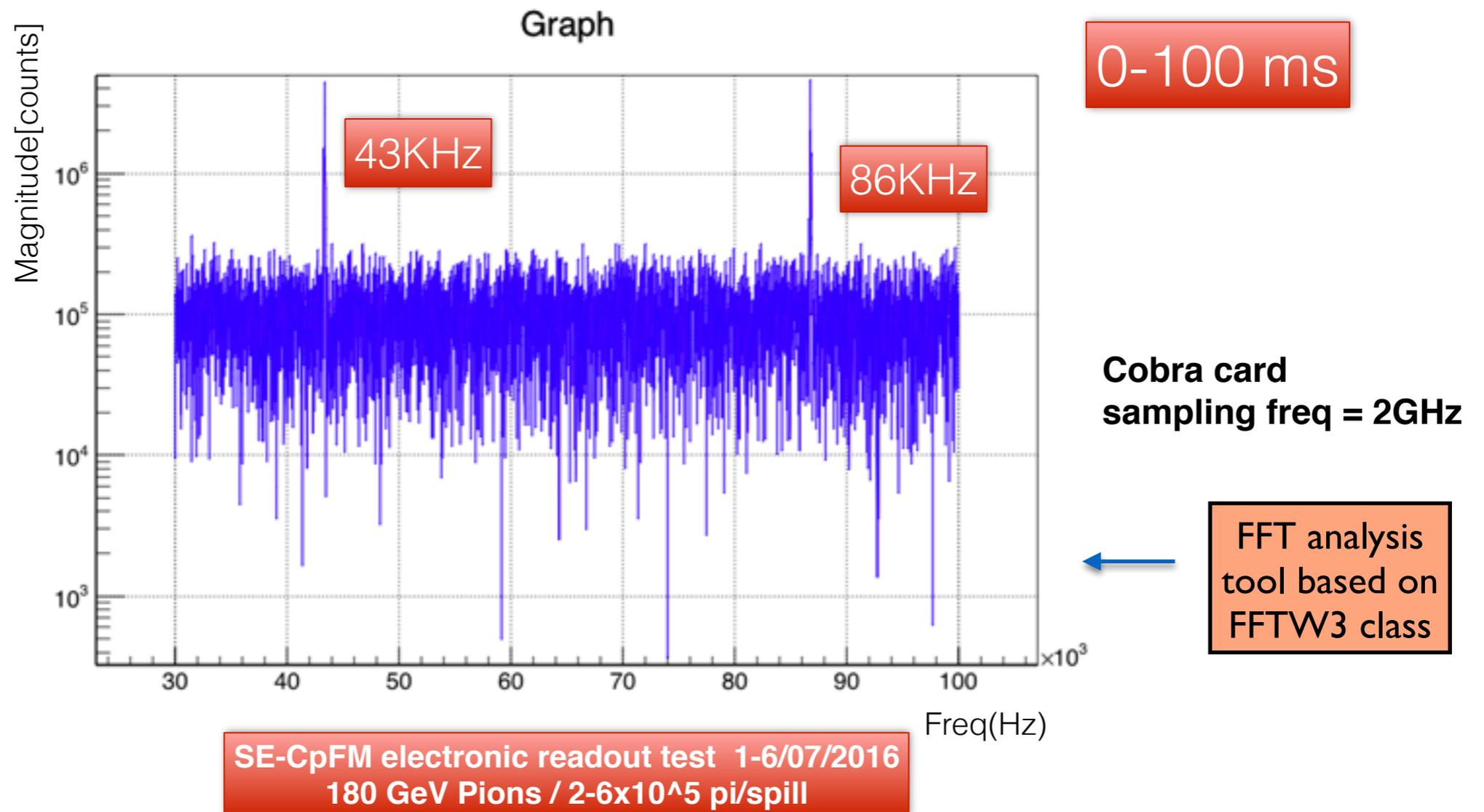
The validation of the Cobra card in terms of Dynamic range is still to be completed. No evidence for the 200 MHz harmonic has been found in H8; we are investigating about it.
