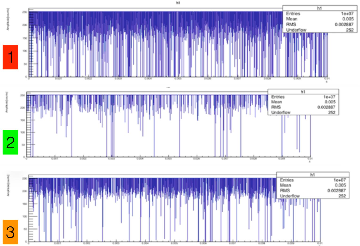
Digitized 10 ms waveforms, corresponding to different pion flux during the same spill.
