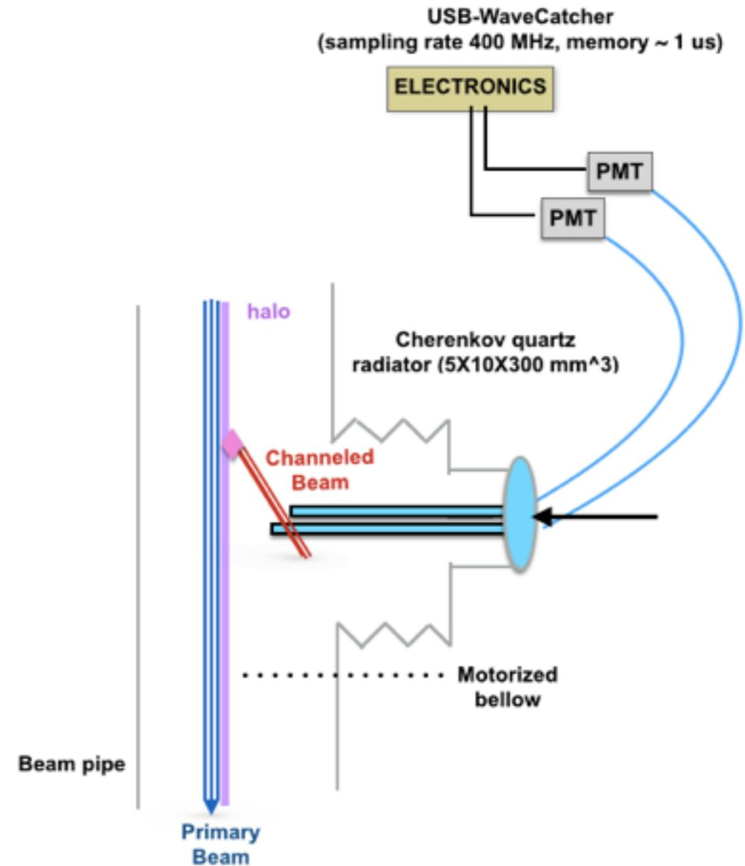
Calibrated at BTF with 500MeV/c electrons:
