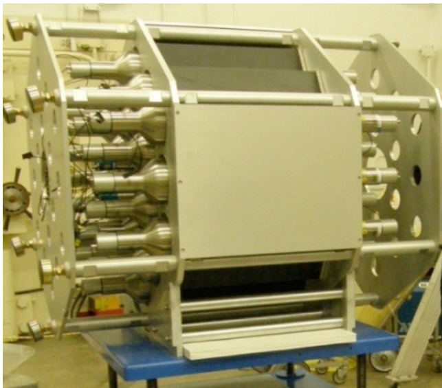
MTAS = Modular Total Absorption Spectrometer
