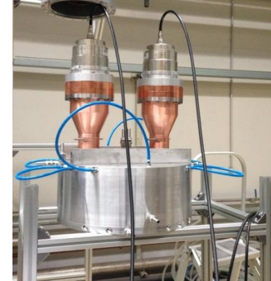
High power RF Coupler 200kW 100% duty cycle
