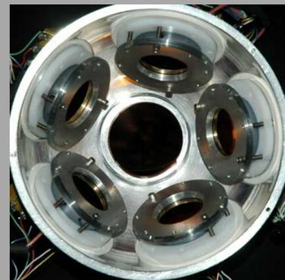
**The  $8\pi$  spectrometer was a world unique device for  $\beta$ -decay studies. Simultaneous collection of  $\gamma$ -singles,  $\gamma\gamma$  coincidences,  $\beta$  tagging, conversion electrons, and lifetime measurements**
