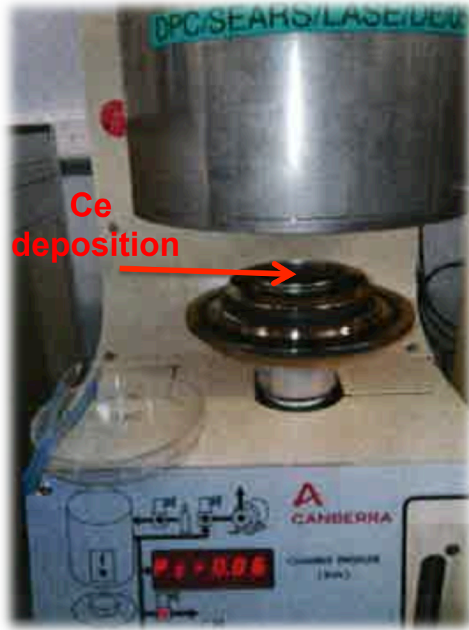
CANBERRA type IN 114, ionization chamber, 100% in 2π st. \sigma_E = 40 keV at CEA/LASE
