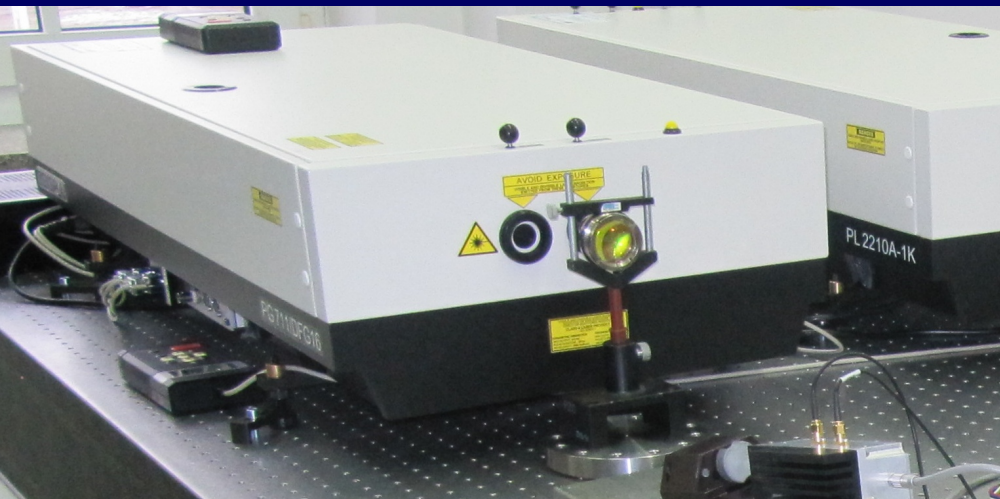
response time with OPO pulses UV to 16 \mu\text{m} , 25 ps pulses, 2 MW
