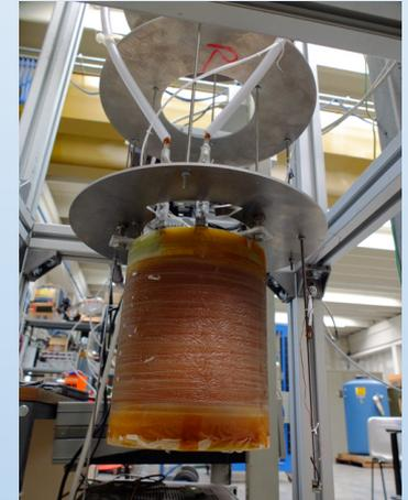
Cryogenic system in Frascati Superconducting magnet
