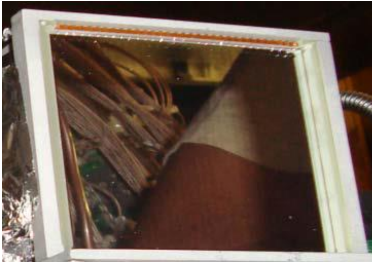
Photograph of one 300 \mu\text{m} thick DSSSD - BB7 design.
