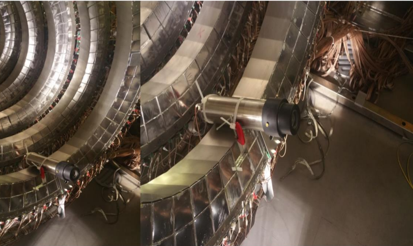
PM -EMI 9954QA Like in ARGOS detector
