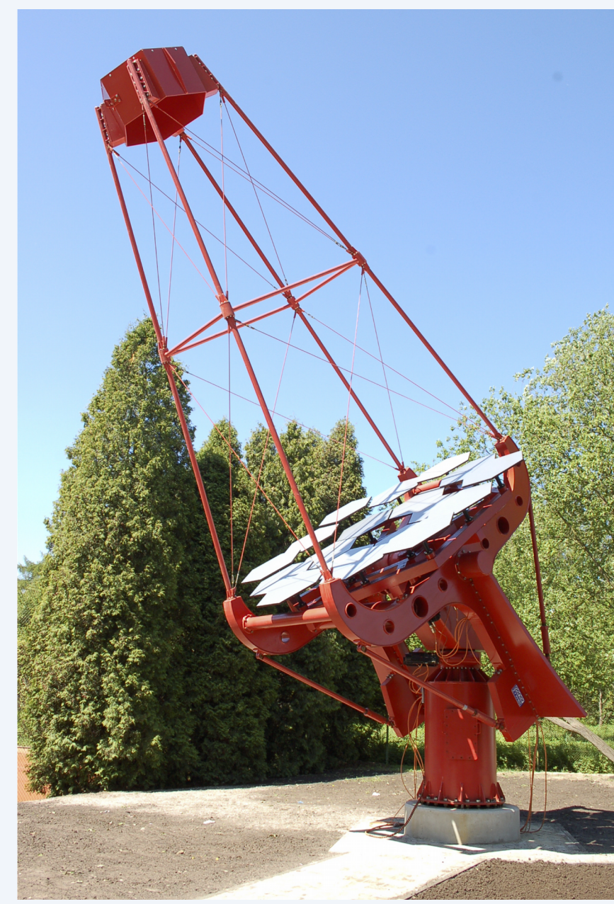
The SST-1M 4-m diameter Davies-Cotton with 9° FoV telescope prototype in Krakow
