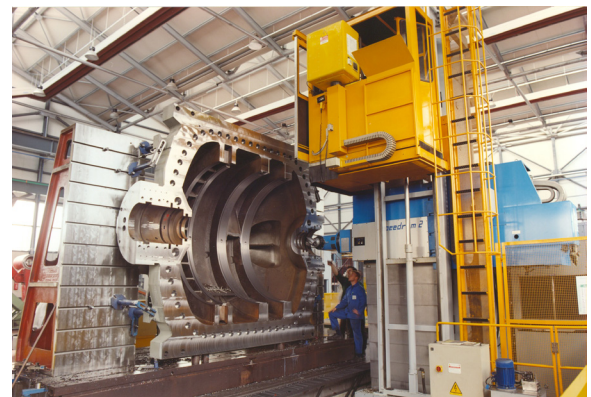
Castellini workshop has top quality machining equipment, large assembly area and testing team. Turbine case during machining.
