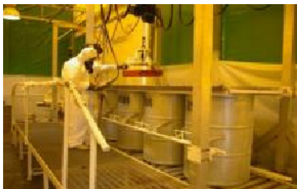
Transportable plant for sorting and supercompaction
