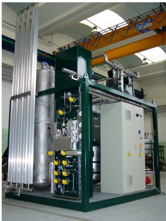
Design and manufacturing of a Skid mounted helium purification system
