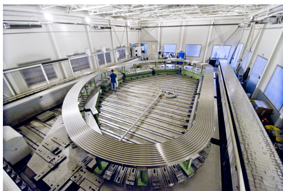
Radial Plate manufacturing-ITER project
