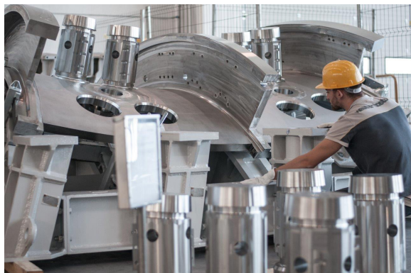
Manufacturing of the Vacuum Vessel sectors for the largest international nuclear fusion project ITER
