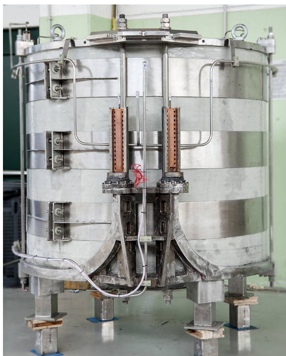
A Nb 3 Sn large bore coil, designed and produced by ICAS for the NAFASSY measurement station at the University of Salerno (IT)
