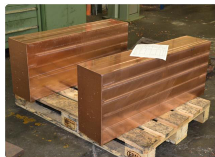
Machined parts in Cu-OFE and CuCrZr
