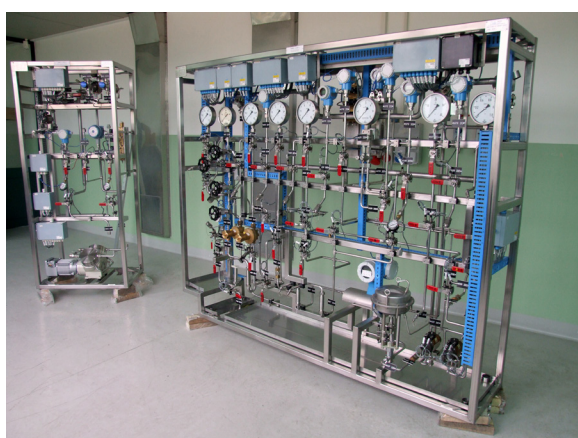
Design and manufacturing in clean area of Gas mixing panels
