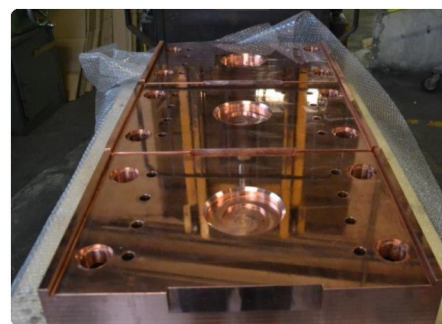
Machined parts in Cu-OFE and CuCrZr
