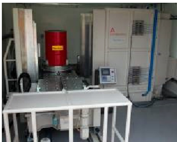
Passive Active Neutron Waste Assay System for Pu and U Assay
