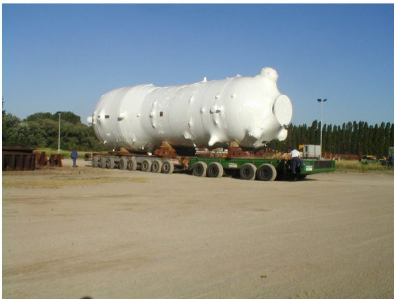
Primary Sodium Pump - Superphénix Nuclear Power Station, Creys-Malville, France
