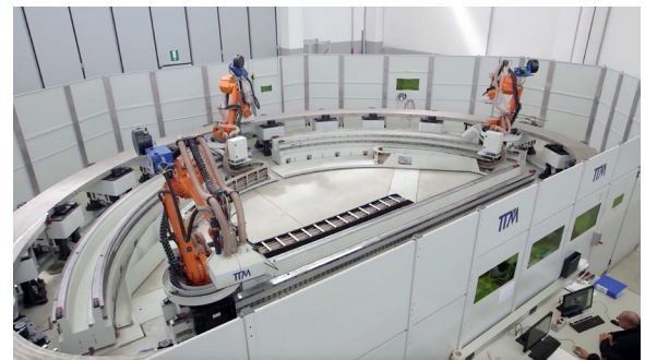
Fully automated process for laser welding of stainless steel inductors for ITER fusion reactor
