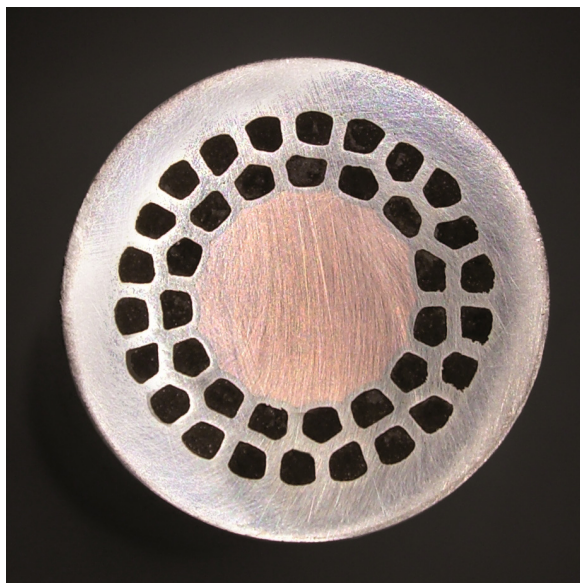
Typical MgB 2 wire cross section
