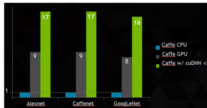
Figure 1: cuDNN performance comparison with CAFFE, using several well known networks. CPU is 16-core Intel Haswell E5-2698 2.3 GHz with 3.6 GHz Turbo. GPU is NVIDIA GeForce GTX TITAN X.
