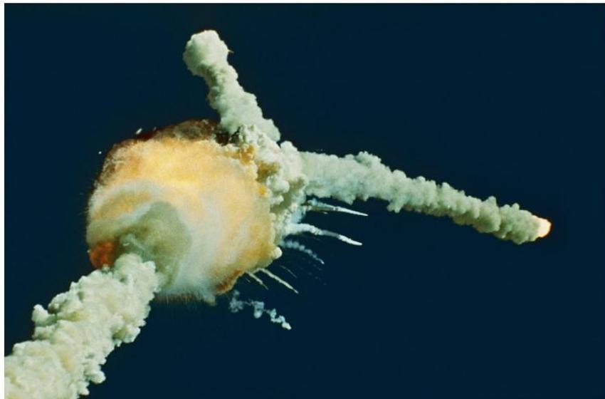
Figure 1: The explosion of Space Shuttle Challenger on January 28, 1986. The primary cause of the disaster was attributed to the failure of an O-ring.
