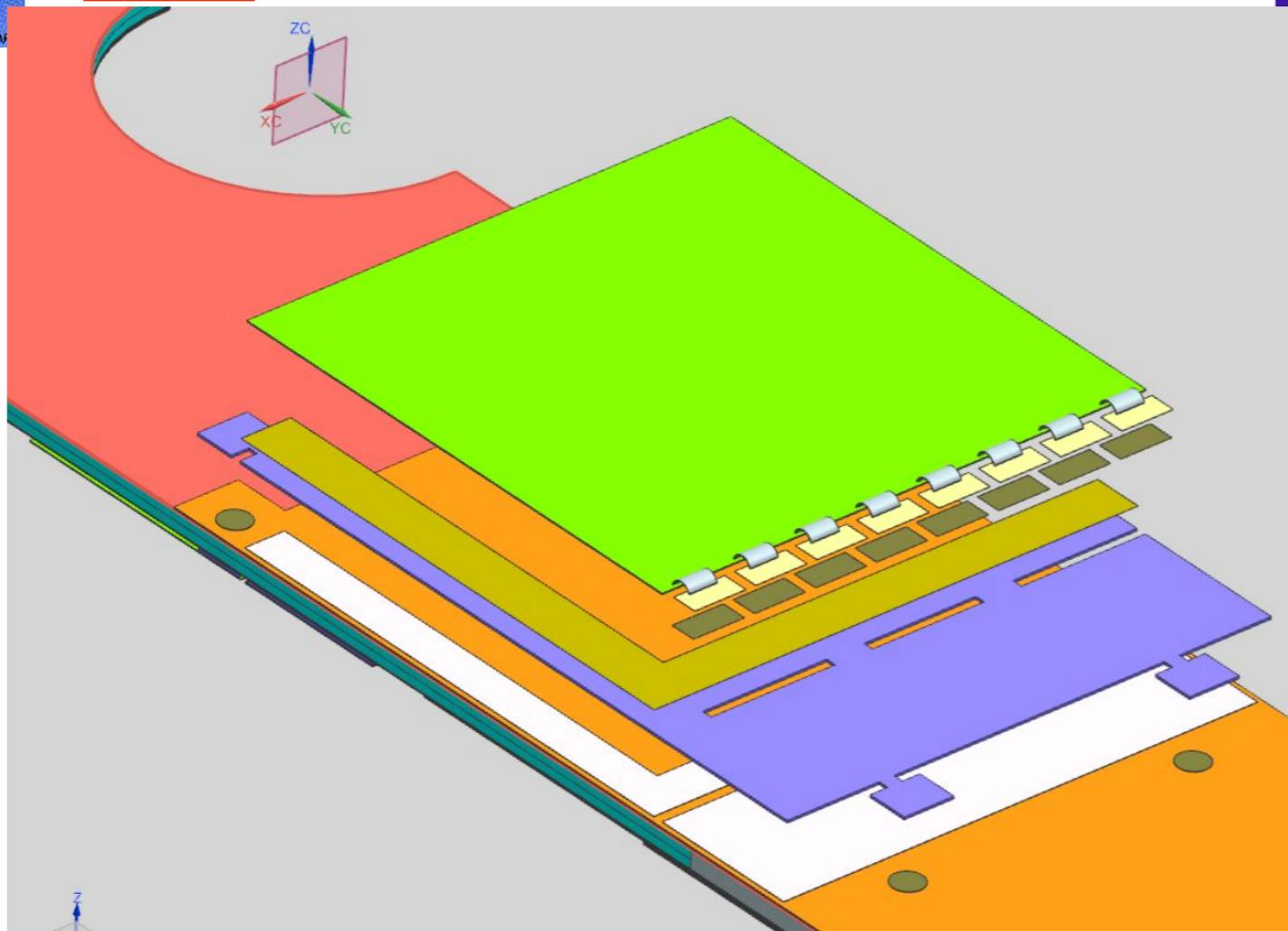
With respect to v5 hybrid solution: no thermal vias, no hybrid flex, no epoxy layer
