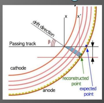
Detector has been aligned using cosmic muon tracks with the magnetic field off
