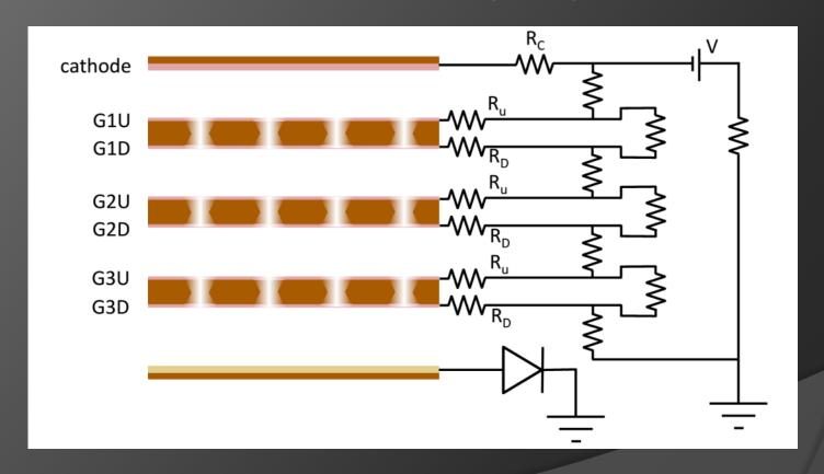
HV passive voltage divider installed to guarantee the safest operation
