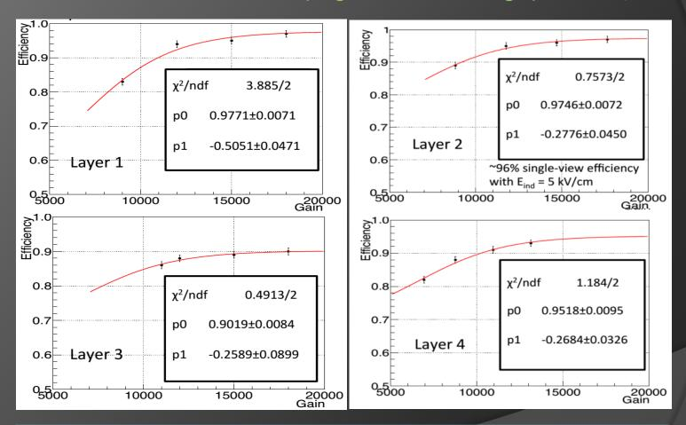
Similar efficiencies are obtained with the new HV voltage divider
