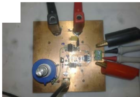
Precision Low Side I Source \mu Ohmetro 4 wires technique
